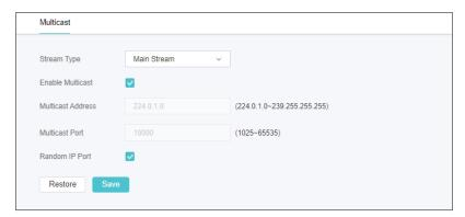
After Multicast enabled, you can watch the video with the URL rtsp://A:B:C:D/multicastStreamN, for example, rtsp://192.168.0.3/multicastStream1. A.B.C.D is the IP address of the camera, and N can be number 1 or 2 that indicates the stream, 1 for main stream and 2 for substream.
