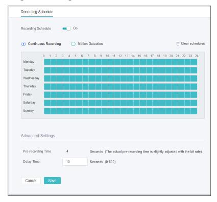
2. Enable Recording Schedule, select continuous recording or motion detection, then select the time.
